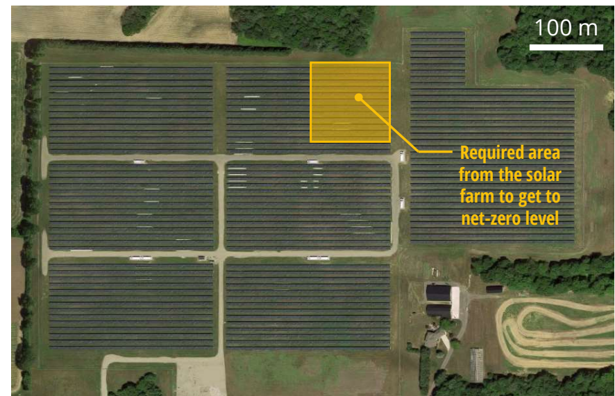
Figure 15: The area of off-site generation required by the development (yellow rectangle) overlaid on the Silvercreek Solar Park, found near Aylmer Ontario (image Courtesy of Google Earth™).
