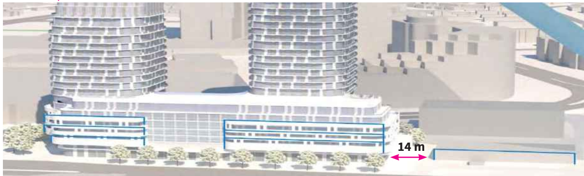
31. North elevation - separation between proposed development and adjacent heritage property. Podium massing is broken down into three massing components that correspond to width of heritage building (Source: WZMH Architects).
